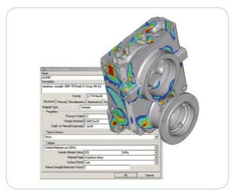
With Pro/ENGINEER Fatigue Advisor, you can easily estimate the number of load cycles your model can sustain before failure.
